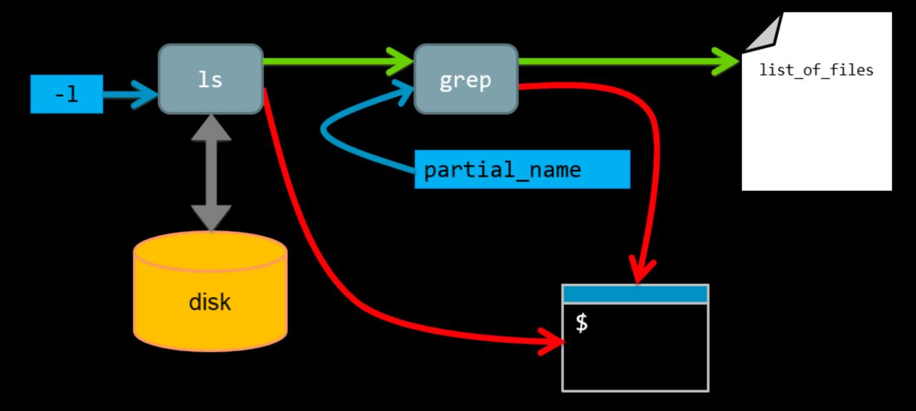
We have **piped** ( ) the **stdout** of one command into the **stdin** of another command!
