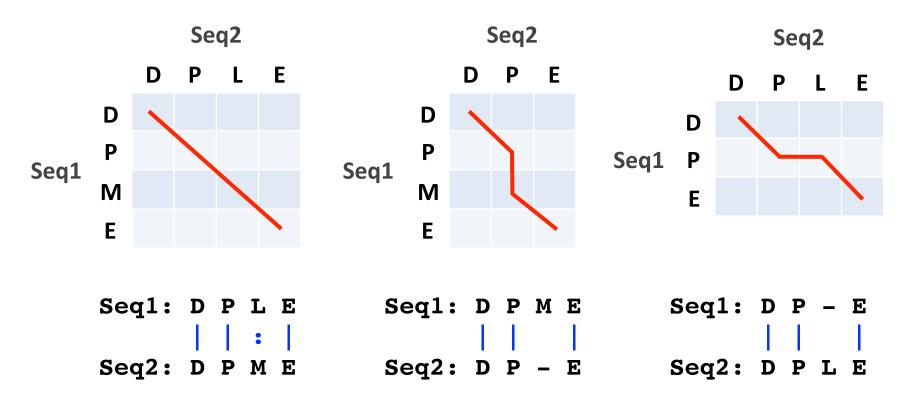
Matches are represented by diagonal paths and indels with horizontal or vertical path segments
